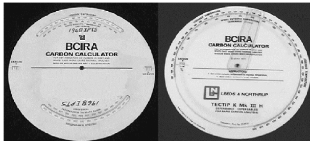
Fig. 6 Two different carbon equivalent calculators
